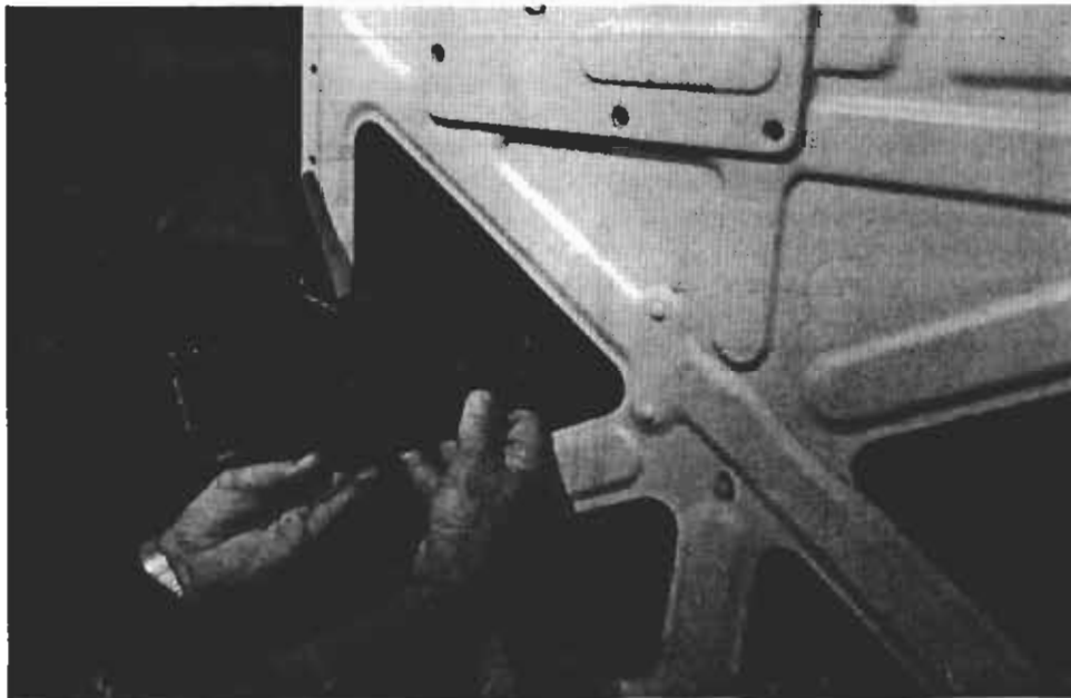
Figure (16) Installation of window regulator through lower forward door opening with riser arms pre-positioned vertically.
